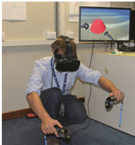
Fig. 7. Preliminary test with user exploring a 3D virtual operational area by HTC Vive.
