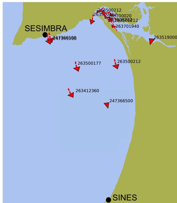
Fig. 2. REP16-Atlantic: Subset of the AIS contacts transmitted delivered to the NRP Arpão submarine operating at depth via JANUS transmissions. Area \sim 60 \text{ km} \times 30 \text{ km}
