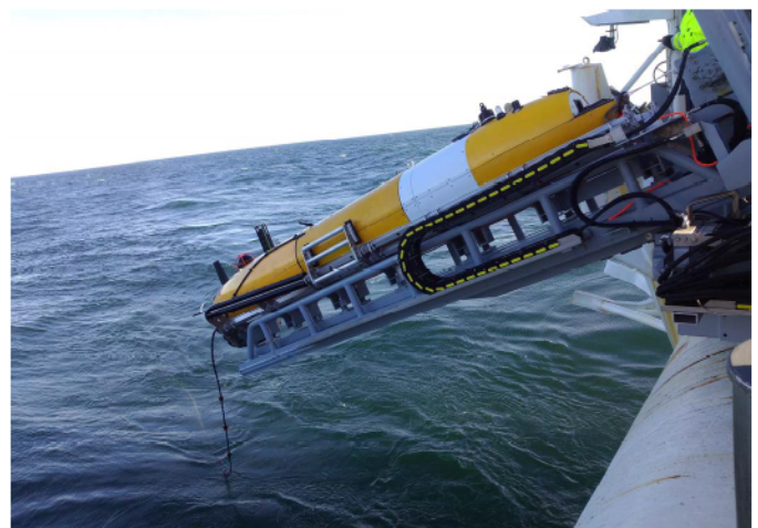
Fig. 12. OEX-C AUV recovered from LARS
