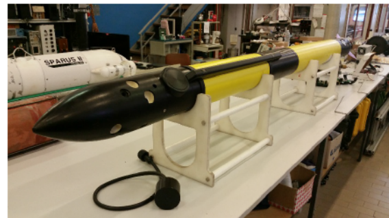
Fig. 3. WPT integration in eFolaga AUV with hockey-puck shaped housing in the AUV and on the bench
