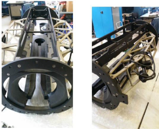
Fig. 5. Dreamcatcher slide-in guide and IPT primary side coil receptacle and dreamcatcher actuator
