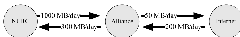
Fig.2: Estimation of data volumes to be exchanged daily during DART06 sea trials
