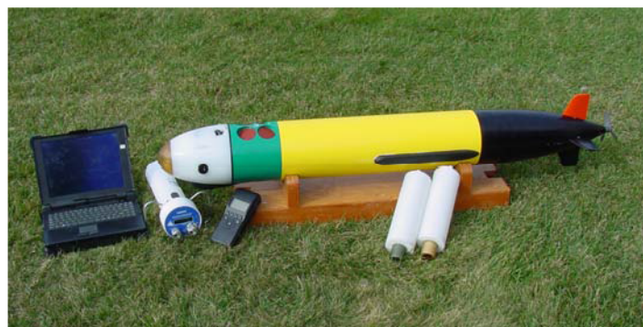
Figure 1 : REMUS vehicle with system components: Notebook, Ranger, handheld GPS, two navigation transponders.
