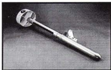
Model 2260NV Instrumented Towfish
