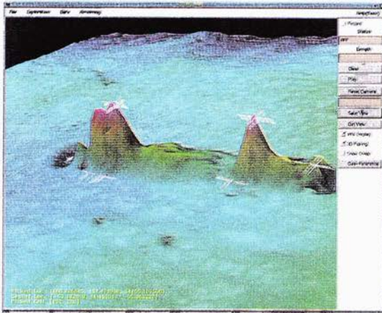
Fig. 7. Single frame from interactive flight through EM-1000 multibeam bathymetry collected over 150 m long wreck of freighter British Freedom outside of Halifax Harbor demonstrating ability to pick, make measurements, and interrogate points in 3-D -- picked points are marked with cross-hairs. Attributes of latest point are displayed in lower left of screen and can be saved to file for later reference.
