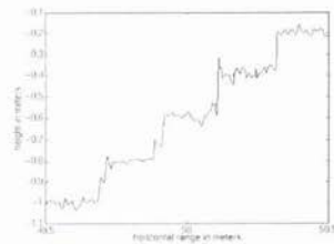
Fig 7. Estimation of STEPS, normalised bandwidth = 0.3
