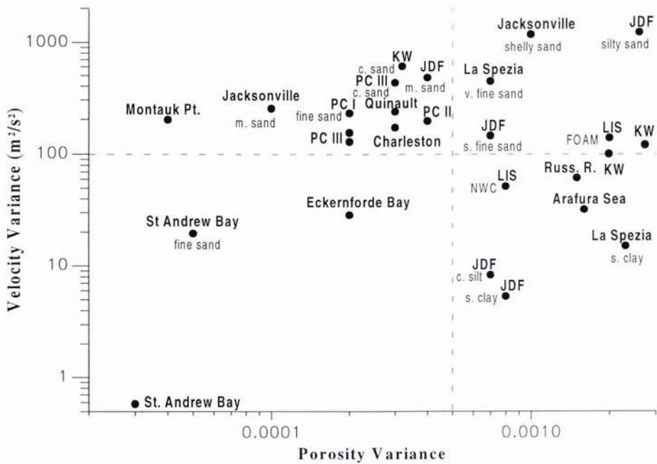
Figure 5: Plot of sediment sound velocity variance vs. sediment porosity variance for various experiment sites investigated.
