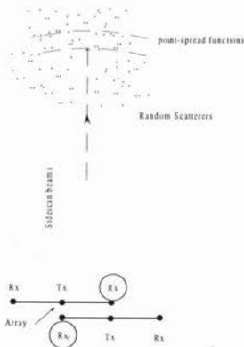
Fig 11. Compare echo from leading Rx, trailing array with trailing Rx, leading array
